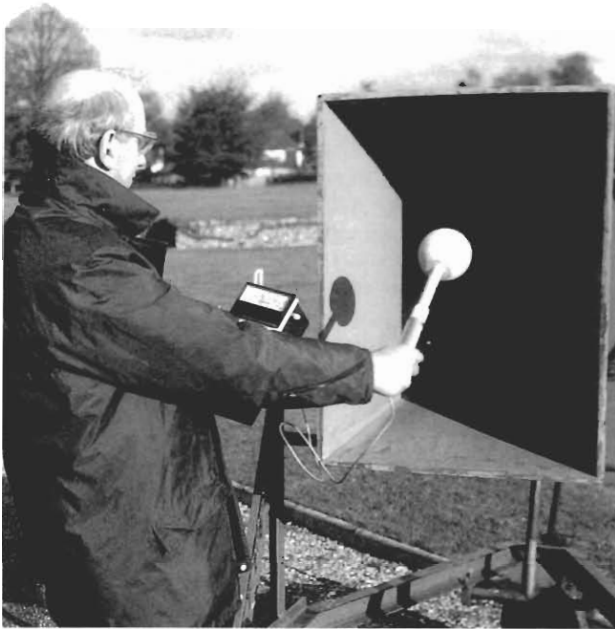
Radiation hazard meters are employed at transmitter sites to measure the RF voltage field. The calibration of the rugged BBC designed ME1/4 hazard meter (right) is being checked in a standard field against a precision laboratory field strength meter (left).
