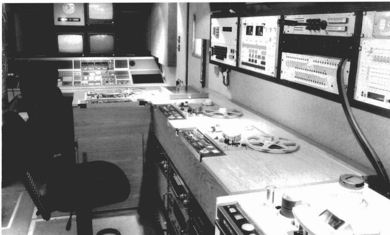
Interior of Television's new Master Sound Control Vehicle (MSC 3)
