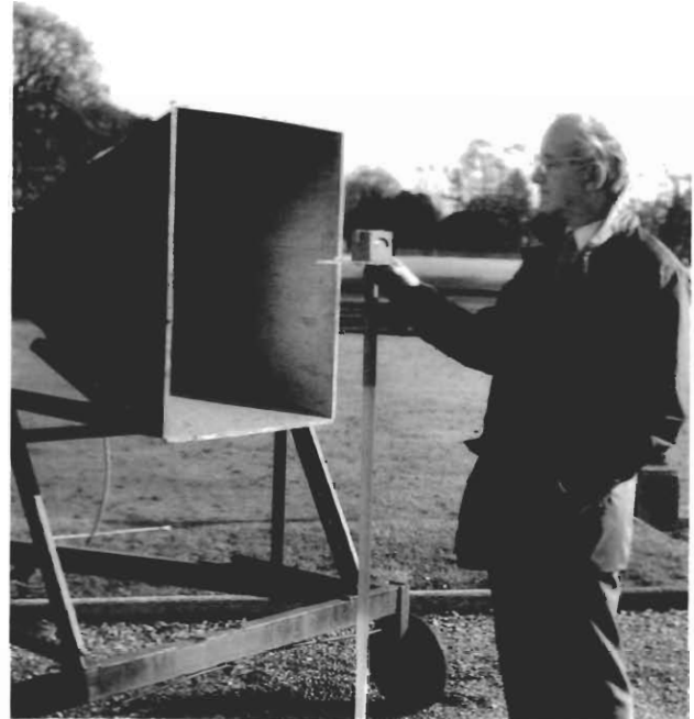
Radiation hazard meters are employed at transmitter sites to measure the RF voltage field. The calibration of the rugged BBC designed ME1/4 hazard meter (right) is being checked in a standard field against a precision laboratory field strength meter (left).
